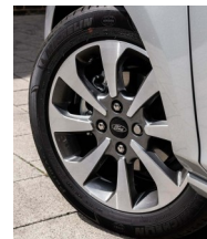
Aluminium/nickel alloy wheel
